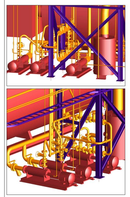
Structural Steel and Platforms as well as Ducting and Large bore Blow-off Pipe was prefabricated in Denmark and Piping was Prefabricated at a workshop in Romania.
