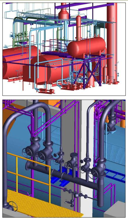
Pictures from a Steam Boiler Plant with LOOS Boilers for a METSO Paper Tissue factory in Algeria. Delivery of Piping, Ducting, Gratings, Cable Tray, Steel Structure, Pipe Supports, Components (Valves, filters, Steam Traps, Platforms (apart from Boiler Top) etc.
