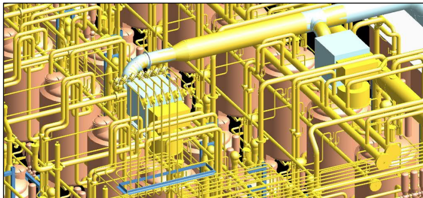
Buffer Preparation Plant @ AGC Biologic ( http://www.agcbio.com ). Process, PID, Sizing, HVAC, Piping and Mechanical Design of the Buffer Prep.
