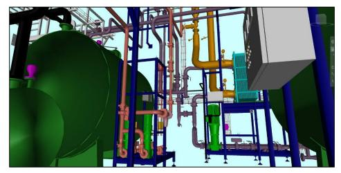
Pictures from a Neutralization Plant in a Pharmaceutical Factory in Denmark. Designed for continuous operation with both pH adjustment and Cooling of Wastewater. Contract performed as EPCm.
