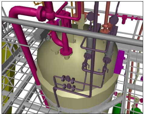
Pictures from a Kill Plant in a Pharmaceutical Factory in Denmark. Designed for 2 off Batch Kill Vessels. No heat recovery and cooled with cooling water based on Client Specification. Contract performed as EPCm.
