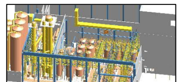
Pictures from a very large Ultrafiltration Installation in Food & Beverage Ingredient – Lactose Production - placed in Germany.
